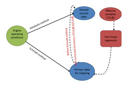
$\textbf{Fig1}. \ \textbf{Schematic of the proposed approach to modeling SE}$
